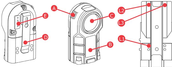
The red L1 light will light up when the power supply is connected, at the same time the L2 and L3 lights will flash.
